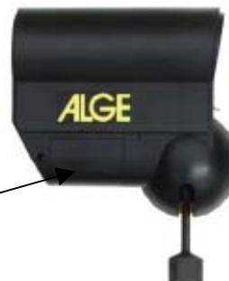
Impulse length of 20 up to 1400 ms adjustable (screw with little screw driver)
